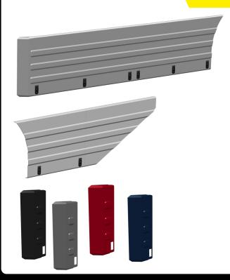
The Parlok Aero panels for sideguard system's function is to reduce the turbulence under and drag behind the trailer by directing the airflow more economically past the trailer. According to CFD simulations and track tests the Parlok sideguard comes up to 13% in drag reduction and over 5% in fuel consumption measured for a combination of towing vehicle with a standard semi-trailer.
